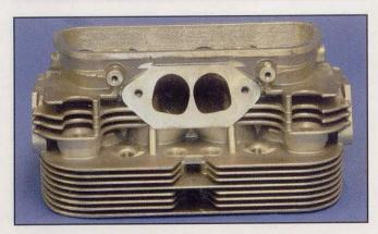
050 casting heads come with as-cast D-intakes and enlarged exhaust ports.
