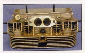
Auto Linea-made 043 head with stock valves and small 12mm plugs.
