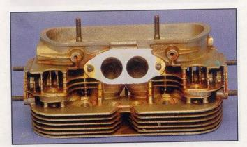
A rare VW head from the past with two less fins and small chambers.
